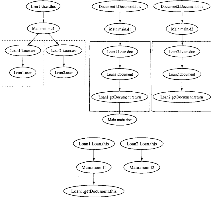
Fig. 2.5. Object sensitive OFG. Dashed (resp. solid) boxes indicate a method body replicated for each allocated object.
